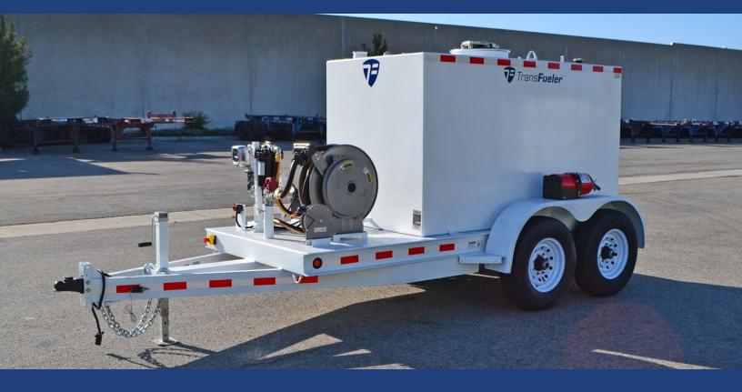
This package features a Double Wall 1,000-gallon tank. It consists of a stainless-steel primary tank with internal baffles and a mild steel outer containment with powder coat finish. It is mounted to a 21K GVW triple-axle steel trailer, is DOT approved for use with JET-A, and can be towed on public highways when full.
