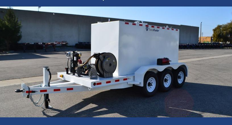
This package features a Double Wall 1,500-gallon tank. It consists of a stainless-steel primary tank with internal baffles and a mild steel outer containment with powder coat finish. It is mounted to a 21K GVW triple-axle steel trailer, is DOT approved for use with JET-A, and can be towed on public highways when full.
