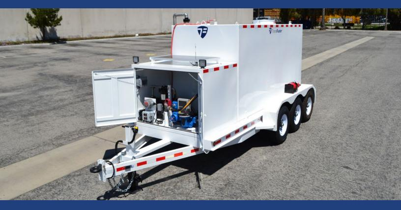
This package features a Double Wall 2,000-gallon tank. It consists of a stainless-steel primary tank with internal baffles and a mild steel outer containment with powder coat finish. It is mounted to a 21K GVW triple-axle steel trailer, is DOT approved for use with JET-A, and can be towed on public highways when full.
