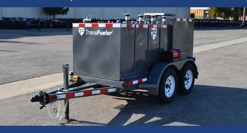
This aviation package features four Single Wall 119-gallon stainless steel tanks. All the tanks are individually baffled and come with locking fill caps, level gauges, rollover vents, and sump valves. Individual shutoff valves allow for precise fuel control and on-road safety. The tanks are mounted on a 7K GVW dual axle trailer, which is DOT-approved for JET-A and can be towed on public highways when full without needing Hazmat.
