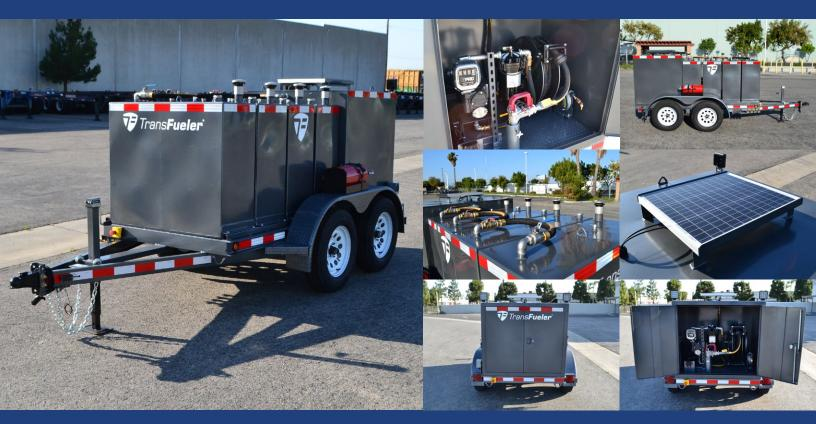
Our standard aviation equipment packages are all made up of proven aviation grade names such as Great Plains Industries, Facet, OPW, Continental Hose, and Hannay. We can customize the equipment packages to run off 12volt DC, 115-volt AC, or a gasoline-powered pump.
