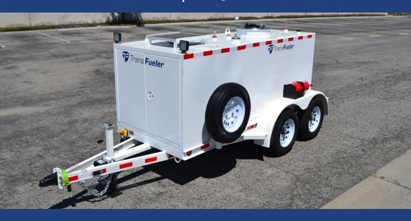
This package consists of a Double Wall 500-gallon tank. The tank has a stainless steel primary tank with internal baffles with a mild steel outer containment tank. The tank is mounted to a 7K GVW dual-axle steel trailer. The trailer is DOT-approved for use with JET-A and can be towed on public highways when full.
