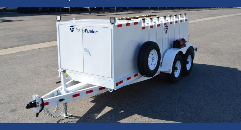
This aviation package features eight single wall 119-gallon stainless steel tanks. All the tanks are individually baffled and come with locking fill caps, level gauges, rollover vents, and sump valves. Individual shutoff valves allow for precise fuel control and on-road safety. The tanks are mounted on a 14K GVW dual axle trailer, which is DOT-approved for JET-A and can be towed on public highways when full without needing Hazmat.
