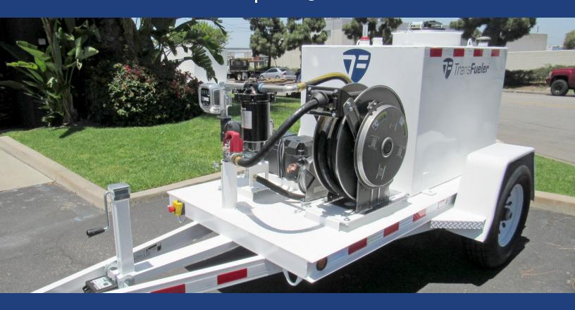
This package features a Double Wall 250-gallon tank. It consists of a stainless-steel primary tank with internal baffles and a mild steel outer containment with powder coat finish. It is mounted to a 3.5K GVW single-axle steel trailer, is DOT approved for use with JET-A, and can be towed on public highways when full.
