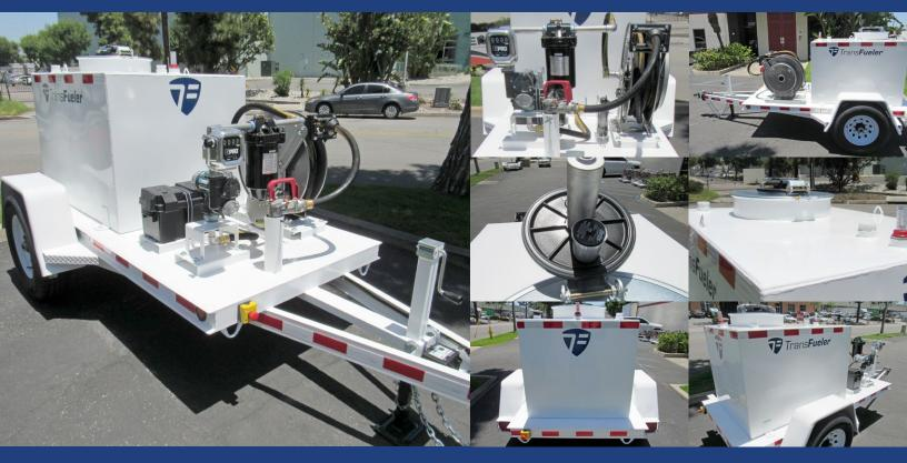
Our standard aviation equipment packages are comprised of 100% aviation-grade components. Featuring the most trusted brands in the aviation industry, such as: Great Plains Industries, Facet, OPW, Continental Hose, and Hannay. We can customize the equipment packages to run off 12 volt DC, 115 volt AC, or a gasoline-powered pump.
