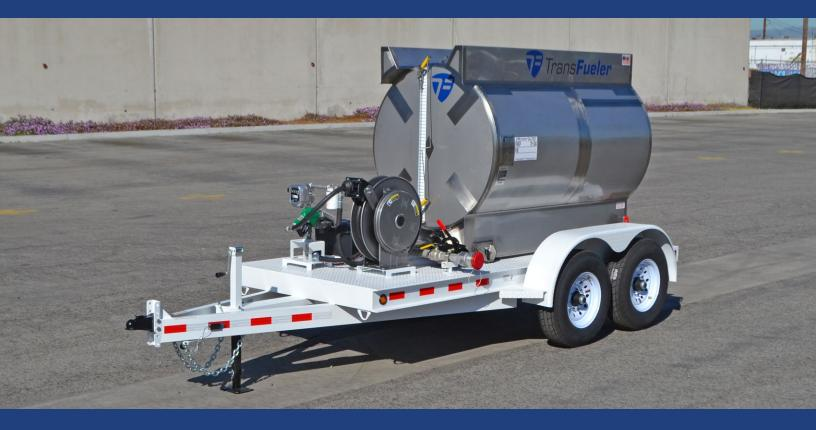
This package includes a 304 Stainless Steel DOT 406 Specification tank mounted on a 7K GVWR dual-axle steel trailer. The trailer is DOT-approved for use with Avgas, Jet-A, JP-8, and other aviation fuels. It can be towed on public highways when full, provided proper Hazmat placards and a commercial driver's license are obtained.
