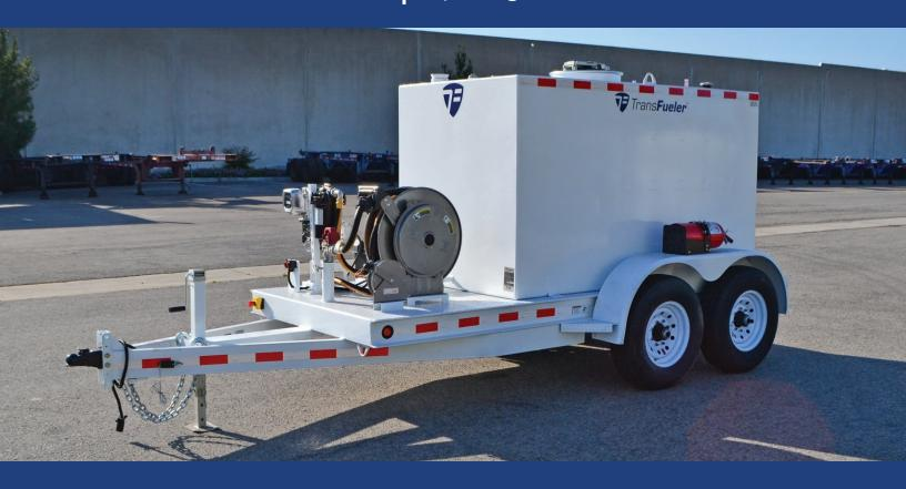
This package features a Double Wall 1,000-gallon tank. It consists of a stainless-steel primary tank with internal baffles and a mild steel outer containment with powder coat finish. It is mounted to a 14K GVW double-axle steel trailer, is DOT approved for use with JET-A, and can be towed on public highways when full.
