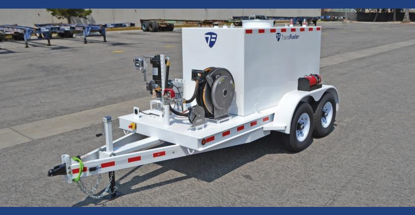
This package features a Double Wall 750-gallon tank. It consists of a stainless-steel primary tank with internal baffles and a mild steel outer containment with powder coat finish. It is mounted to a 14K GVW double-axle steel trailer, is DOT approved for use with JET-A, and can be towed on public highways when full.
