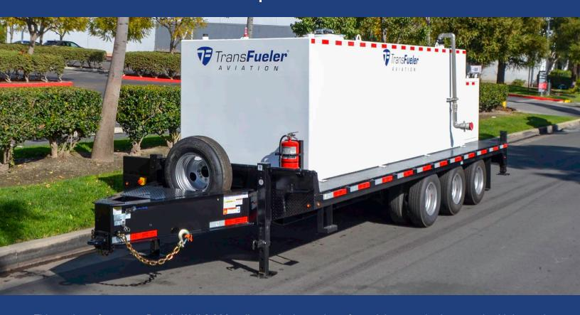
This package features a Double Wall 3,000-gallon tank. It consists of a stainless-steel primary tank with internal baffles and a mild steel outer containment with powder coat finish. It is mounted to a 36K GVW triple-axle steel trailer, is DOT approved for use with JET-A, and can be towed on public highways when full.
