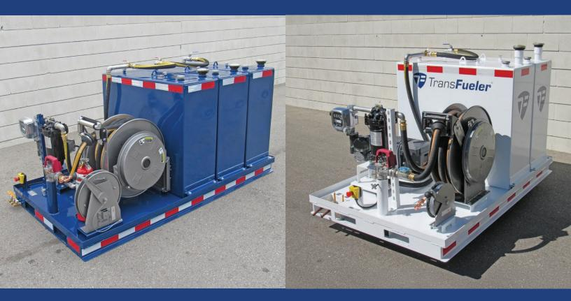
This aviation package features (1, 2, 3, or 4) single wall 119-gallon stainless steel tanks. All the tanks are mounted on a heavy-duty steel platform and can be easily moved using built-in forklift pockets. The M-Series skids can be securely installed on a truck or trailer and are fully compliant for transporting Jet-A fuel on public roads—no Hazmat certification required.
