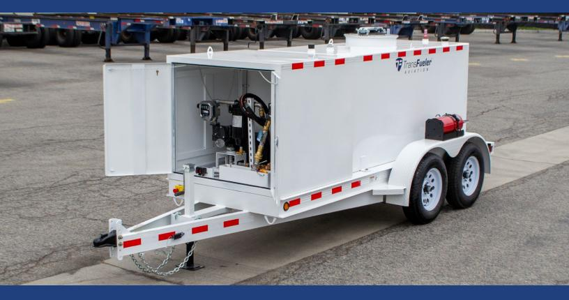
This package features a Double Wall 600-gallon tank. It consists of a stainless-steel primary tank with internal baffles and a mild steel outer containment with powder coat finish. It is mounted to a 14K GVW double-axle steel trailer, is DOT approved for use with JET-A, and can be towed on public highways when full.
