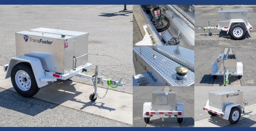
Our standard aviation equipment packages are comprised of 100% aviation-grade components. Featuring the most trusted brands in the aviation industry, such as: Great Plains Industries, Facet, OPW, Continental Hose, and Hannay. Dispensing equipment packages run on 12-volt DC, 115-volt AC, or a diesel/gas powered pump.
