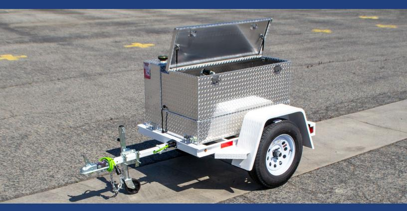
This package includes a diamond plate aluminum tank with a storage box mounted on a 3.5K GVWR single-axle steel trailer. The trailer is DOT-approved for use with Avgas, Jet-A, JP-8, and other aviation fuels. It can be towed on public highways when full.
